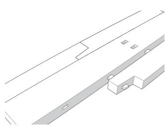
Figure 5.3 A simple model of bottom plank structure showing *jangsaks*. (Drawn by Randall Sasaki)
