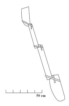
Figure 5.11 A cross-section diagram of the Taean ship's plank arrangement. (Reproduced by Randall Sasaki from Munhwajaechung Guklip Haeyang Munhwajae Yeonguso 2009)
