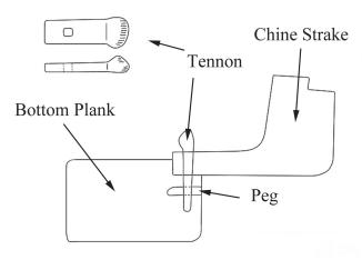
Figure 5.10 A drawing showing a joining configuration of bottom plank and the L-shaped chine strake. (Drawn by Randall Sasaki)
