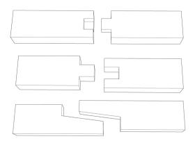
Figure 5.7 Example of some of the joinery found in Korean vessel. Top: complex tongue and groove joint, Middle: square tongue and groove joint, Bottom: step joint. (Drawn by Randall Sasaki)
