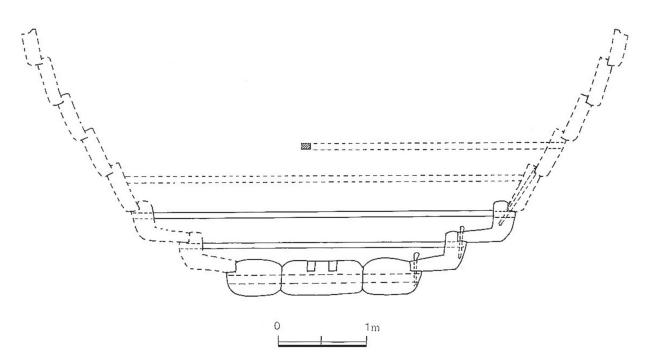
Figure 5.5 A possible reconstruction drawing of Sibidongpado ship. (Courtesy of the National Research Centre of Marine Cultural Heritage)
