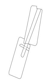
Figure 5.4 A simple drawing showing *pisak* and plank configurations. (Drawn by Randall Sasaki)
