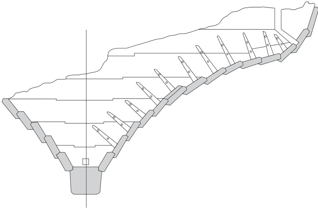
Figure 49. Shinan Ship cross-section of the Shinan Ship.
